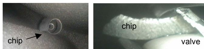
Figure 2: Chips lodged in cylinder block water jacket [Friedrich, 2004] and cylinder head oil valve [Reich-Weiser, 2006].
