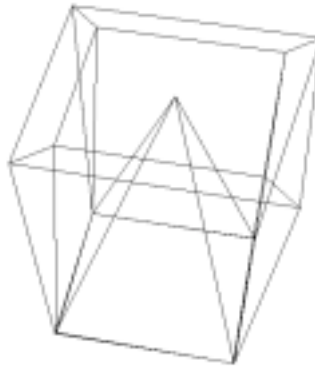
Figure 7.19: For this pseudo-2-manifold part (a pyramid inside a toroidal frame), a slice through the very bottom will consist of three coincident contours: two outer contours and one inner hole contour. Here we do have material; we output an outer contour.
